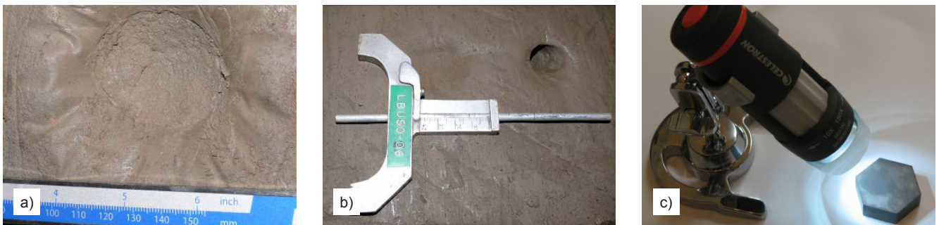
Figure 4. Sample evaluation; a) trauma depth evaluation, b) trauma depth measuring device, c) celestron digital microscope.
