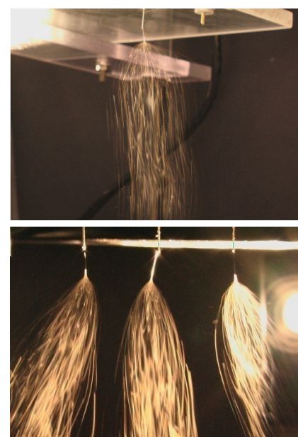
Figure 2. Single nozzle and multinozzle electrospinning plumes (PVDF for non-woven mat production) - exposure 1/50 s)
