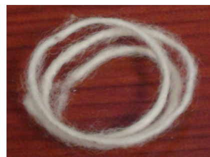
Figure 7. SMA CSFY actuated into a spiral shape.
