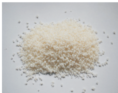
Figure 2. Hue of co-polyester granulate made with a modifying additive.
