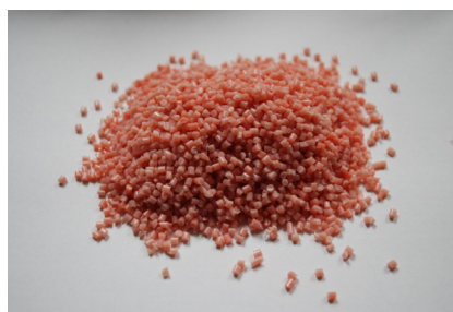
Figure 1. Hue of co-polyester granulate made without the modifying additive.
