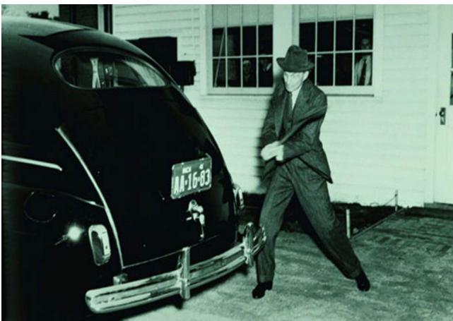
Figure 6. One of the most famous photographs (1941) of Henry Ford who is trying to crack a rear deck lid composed of paper and soybean resin with a sledge hammer.
