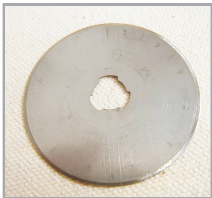
Figure 1. Blade used in cut resistance tests according to standard A.
