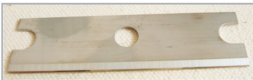
Figure 2. Blade used in cut resistance tests according to standard B.
