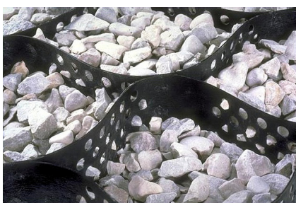
Figure 2. Cellular geonet filled with aggregate – ex ample[3].
