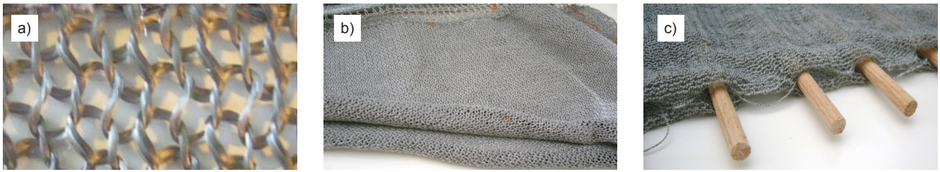
Figure 2. The knit shielding structures: (a) face view of the left-right knit structure (I) made of 100% steel filaments, and (b) view of the double knit structure (II) made of left-right stitch, the structure has the form of sleeve without connections between sides (layers), and (c) view of double structure III with internal tunnels. Two separate fillings were introduced into the tunnels, which can be observed as loose threads. Wooden sticks were also introduced into the tunnels to make these spaces more visible in the picture.
