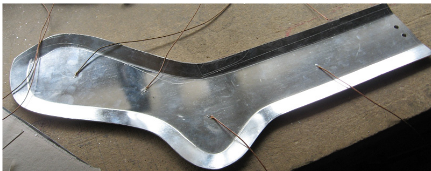
Figure 1. Places of thermo receptors in the hot unit.
