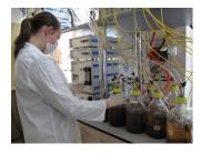
continuous reading of the  $\mbox{ CO}_2$  delivered. The laboratory's modern MICRO-OXYMAX RESPIROMETER is used for carrying out tests in accordance with International Standards.
