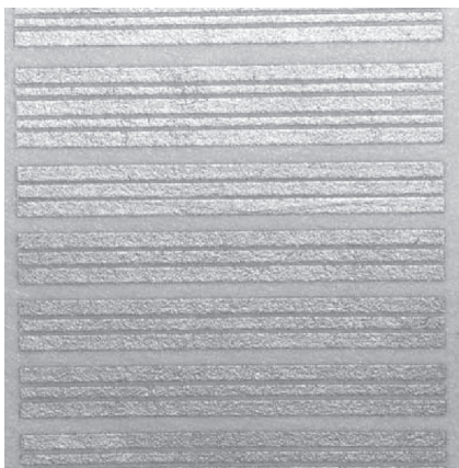
Figure 2. Textile transmission lines deposited by the printing method [7].
