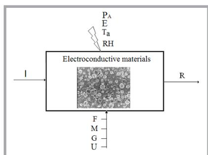
**Figure 3.** Qualitative model of resistance measurement of a textile electrode;  $I$  – current,  $R$  – resistance;  $F$  – pressure force,  $M$  – kind of material,  $G$  – geometrical size of a textile electrode,  $U$  – measuring voltage,  $P_A$  – atmospheric pressure,  $E$  – electromagnetic interference,  $T_a$  – ambient temperature,  $RH$  – relative humidity.
