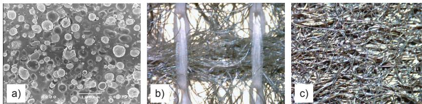
**Figure 2.** Microscopic photos of electroconductive materials tested; a) silicone foil, b) Woven fabric plain weave, c) nonwoven.
