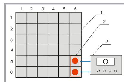
**Figure 4.** Simplified scheme of a stand for measuring surface resistance; 1 – textile electrode, 2 – dual point probes, 3 – Agilent 6.5 Digits Mullimeter.
