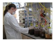
continuous reading of the  $\,\text{CO}_2$  delivered. The laboratory's modern MICRO-OXYMAX RESPIROMETER is used for carrying out tests in accordance with International Standards.
