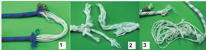
Figure 6. Examples of damage to lanyards. Notes: conditions of performance tests: K3; h = 2.5 m; A = 0.0 m; 1 - lanyard made of TRUST type mountaineering dynamic rope, 2 - lanyard made of type PA12-A-Z/K6/200 fibre rope, 3 - lanyard made of PRO-STATIC type mountaineering static rope.
