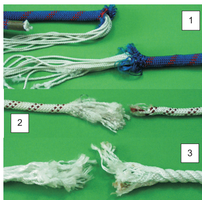
Figure 8. Examples of damage to lanyards. Notes: conditions of performance tests: K1; h = 1.0 m; A = 1.0 m; 1 - lanyard made of TRUST type mountaineering dynamic rope, 2 - lanyard made of PRO-STATIC type mountaineering static rope, 3 - lanyard made of type PA12-A-Z/K6/200 fibre rope.
