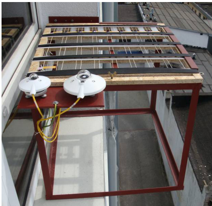
Figure 1. Test stand with frames for sun-light exposure.
