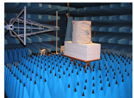
Figure 3. Isotropic spherical generator enclosed with a sample of woven/knitted fabric spread out on a foamed PS cylinder.
