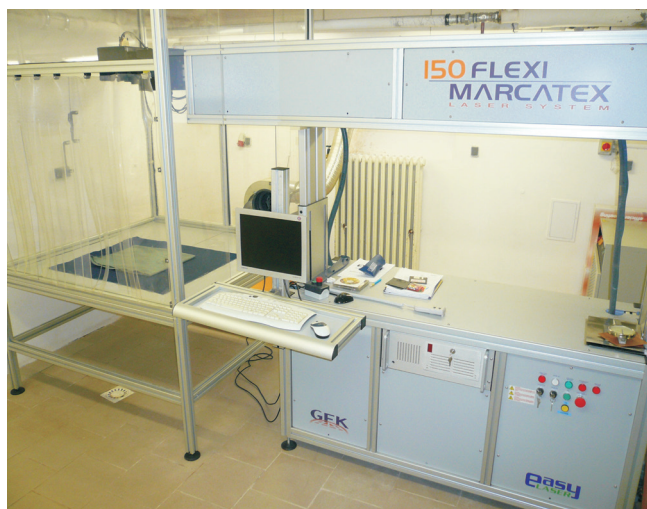
Figure 1. Marcatex laser - used for the thermal stress of the substrate.
