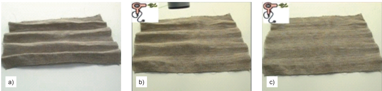
Figure 10. Wrinkle recovery for sample H4 after time period; a) t = 0 s, b) t = 8 s, c) t = 23 s.
