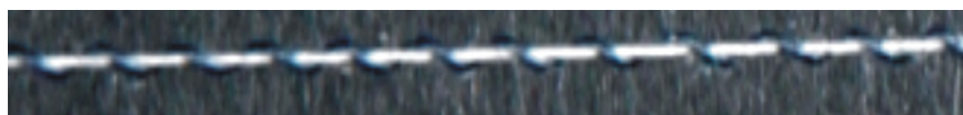
Figure 5. Two-component wrapped fancy yarn (photo taken as the yarn was being produced on a ring twisting machine, in the zone between the twisting cone and the guide positioned just over the spindle. Own research).
