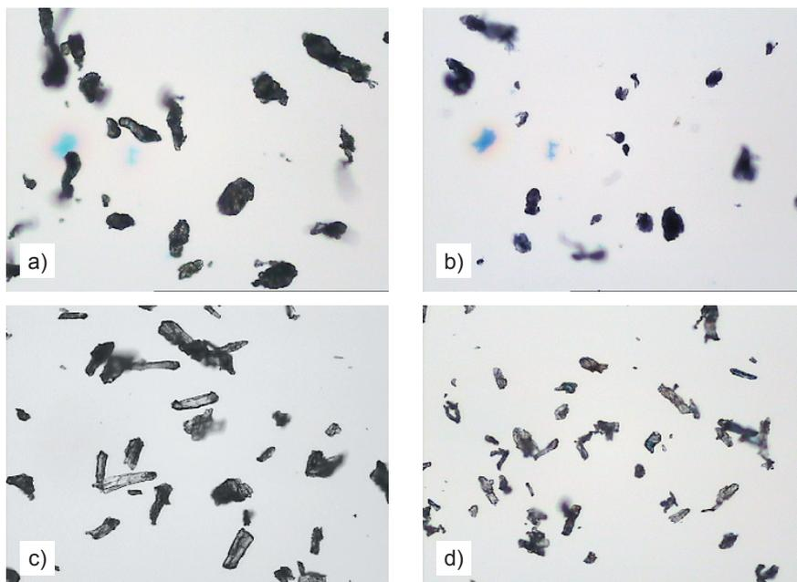
**Figure 4.** Microscopic images of crystallite aggregates of MCC samples: a) MC/R-15/AS-23, b) MC/R-50/AS-21, c) Vivapur 101, d) Vivapur 105.
