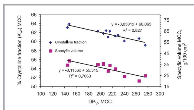
**Figure 2.** Dependence of crystalline phase content and specific volume of MCC on its average polymerisation degree.
