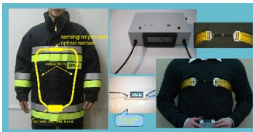
Figure 11. The prototype of the implemented breathing frequency system (BFS).
