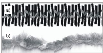
Figure 1. Chenille yarn; a) Chenille yarn structure, b) Chenille yarn picture.
