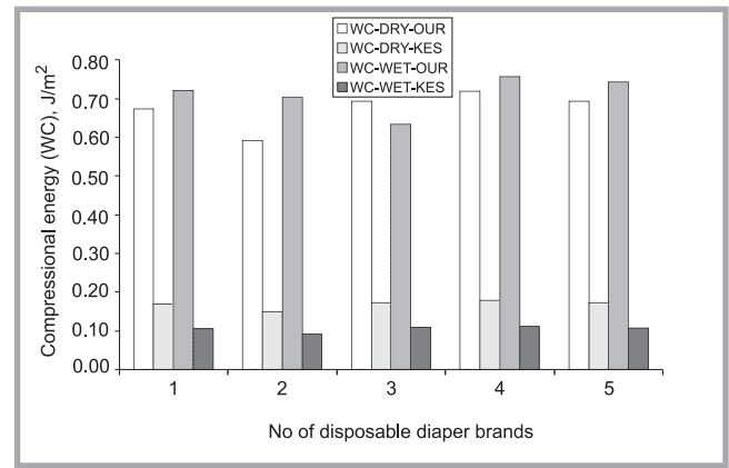
Figure 6. Compressional energy (WC) values of 5 wet and dry commercial diapers obtained from KES and our methods.
