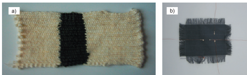
Figure 2. a) knitted sample of sensorial material; b) woven sample of sensorial material with conductive yarns.
