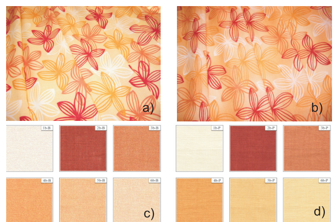
Figure 4. Design »b« printed digitally using ink-jet printing (a) and the same design printed using rotary screen printing (b), color table printed using ink-jet printing (c) containing samples: 1b-B, 2b-B, 3b-B, 4b-B, 5b-B, 6b-B, color table printed using rotary screen printing (d) containing samples: 1b-P, 2b-P, 3b-P, 4b-P, 5b-P, 6b-P [15].
